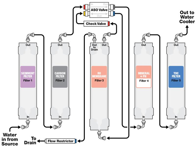
**Sediment filter** removes large contaminants and dissolved solids larger than 10 microns like rust, dust, clay, and pipe residue. (Certified to NSF/ANSI standard 42 for Material Safety)
