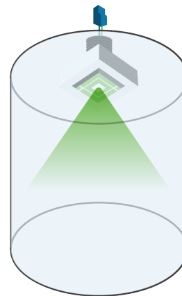
Figure 3: The type of ultraviolet bulb found in many filtered water coolers.
